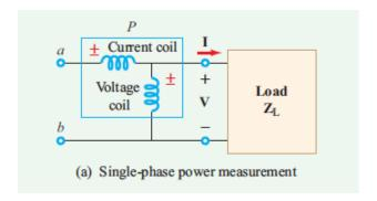
▶ If the  $\pm$  terminal of the current coil is on the end toward the source and the  $\pm$  terminal of the voltage coil is connected to the line in which the current coil is inserted, the calibrated deflection on the wattmeter (or digital display) is equal to the average power P absorbed by the load.  $\blacktriangleleft$
