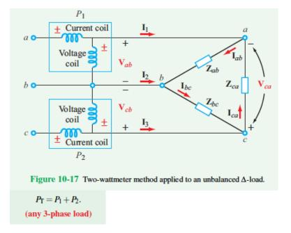
where  $P_{\rm T}$  is the total average power absorbed by any three-phase load (Y or  $\Delta$ , balanced or unbalanced).
