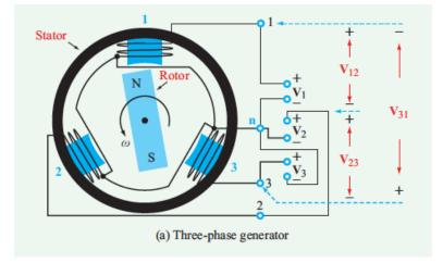
The Y-source configuration has a neutral reference terminal and all three voltages are measured relative to that terminal, such as between terminals 1 and *n* in the figure. In the  $\Delta$  configuration the three voltages are measured between pairs of coils, such as between terminals 1 and 3 in the figure.
