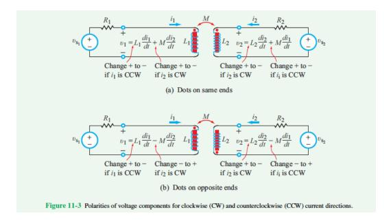
For dots on same ends and currents entering coils at dotted ends (Fig. 11-3(a)):
