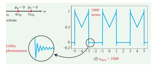
The Fourier series provides an exact representation of a periodic function if the series contains an infinite number of terms. For most waveforms, a finite number of terms is sufficient to provide a good approximation, but if the waveform has discontinuities, the finite (truncated) series exhibits the Gibbs phenomenon (in the form of oscillations) at edges and discontinuities.
