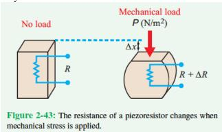
Compression along current direction increases cross-sectional area and reduces length. Hence, compression reduces resistance.
