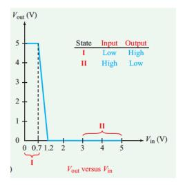
A digital inverter converts a high voltage (representing digital 1) into a low voltage (representing digital 0), and vice versa.
