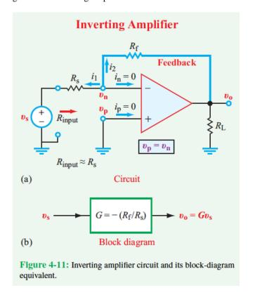
The magnitude of the gain is directly proportional to the feedback resistance  $R_f$ . Maximum feedback means  $R_f = 0$ , in which case G goes to zero, and minimum feedback means  $R_f$  is an open circuit, in which case the gain becomes infinite (but the output cannot exceed  $V_{cc}$ ).
