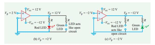
When  $V_p = +2$  V, the op amp causes the red LED to emit light. Switching to  $V_p = -2$  V causes the red LED to stop emitting and the green LED to start emitting.
