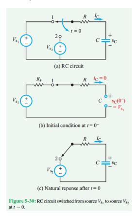
Since the new voltage is lower, the capacitor will need to loose charge. Hence,  $i_C$  in Fig. 5-30(c) should be counterclockwise.
