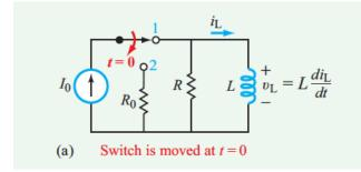
It will flow through R because the current through an inductor cannot change instantaneously.
