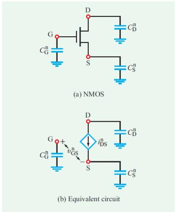
**Figure 5-48:** n-channel MOSFET (NMOS): (a) circuit symbol with added parasitic capacitances and (b) equivalent circuit. [In a PMOS, parasitic capacitances  $C_{\rm D}^{\rm p}$  and  $C_{\rm S}^{\rm p}$  should be shown connected to  $V_{\rm DD}$  instead of to ground.]
