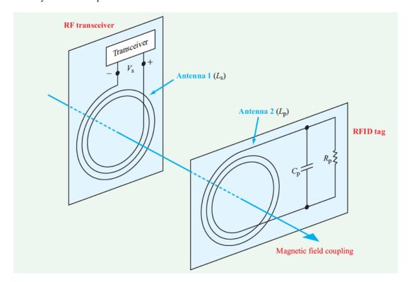
The RFID transfers power through the magnetic field coupling the two coil antennas. These two inductors behave like an air-gap transformer: a sinusoidal current flowing through one coil induces a current in the other.
