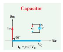
For a capacitor, phasor current is at 90 degrees ahead of the phasor voltage.
