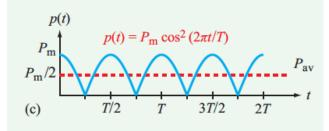
A constant value of  $\phi_1$  or  $\phi_2$  simply shifts the waveforms along the *t* axis. Since the integrations are over a full period, the integrated area is always the same.
