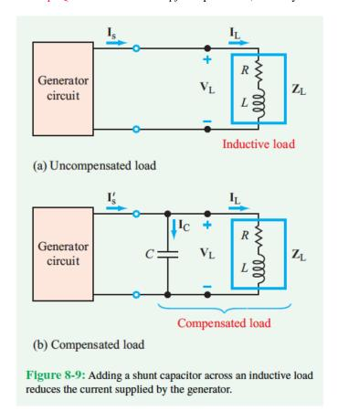
pf compensation refers to increasing the power factor to a value closer to 1. For an inductive load, pf compensation is accomplished by adding a shunt capacitor in parallel with the load.
