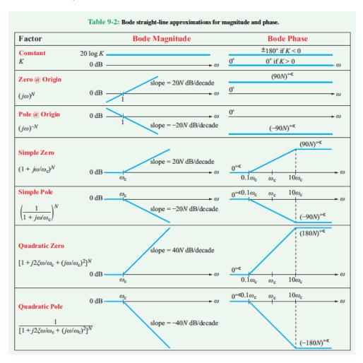
The Bode plots are identical to the exact plots for only the top three in the above table. For the others, the exact plots exhibit continuous change, instead of straight-line approximations, at the corner frequencies.
